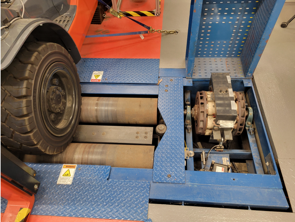
Figure 3: Example of an eddy current dynamometer, as used by MAE 4272 in the Forklift lab. A forklift is not only significantly larger and heavier than the Chicken Coupe, but undergoes very different load cases.
